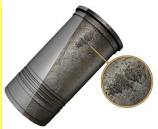
Photo: Case Cylinder liner cavitation erosion
